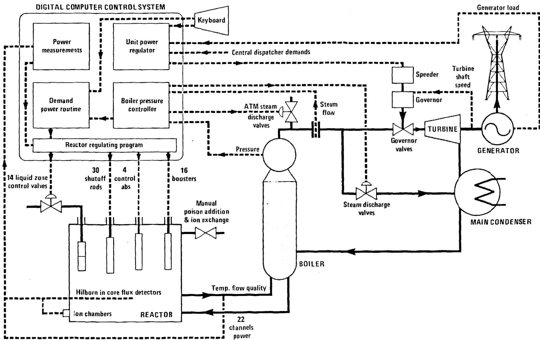
FIG. 6.7: Diagrammatical representation of a reactor control system.
