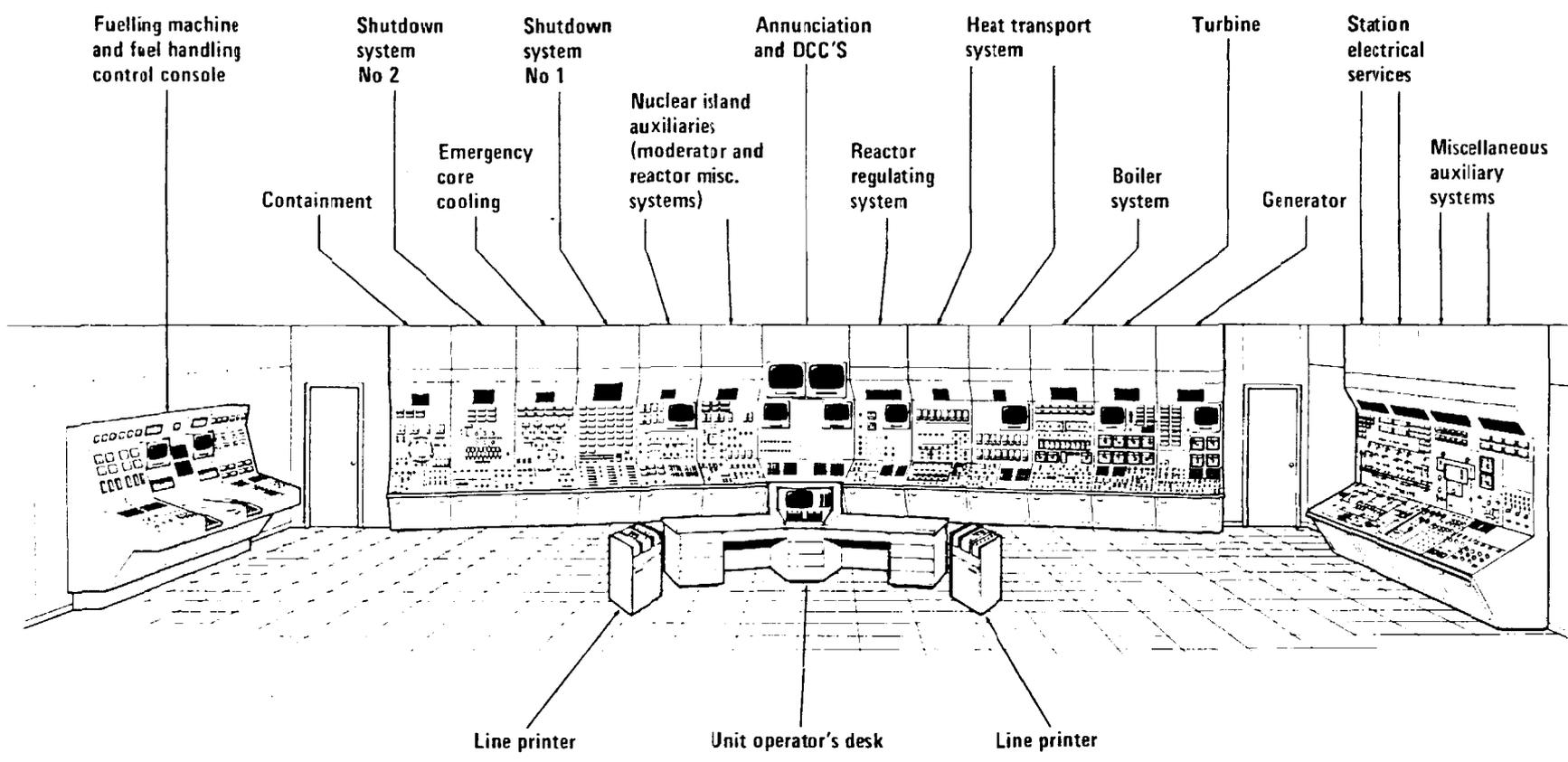
FIG. 6.8: Typical control panel layout.
