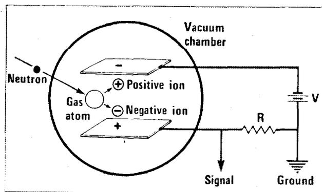
FIG. 6.1: Basic components of an ion chamber.
