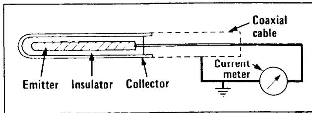
FIG. 6.2: Components of a self-powered (Hilborn) neutron detector.
