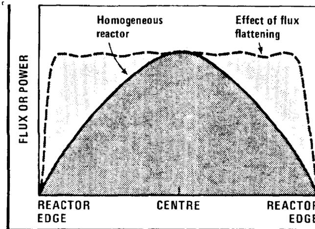
FIG. 6.4: Comparison between a peaked neutron flux associated with a homogeneous core and a flattened flux obtained by the suitable use of flux flattening options.
